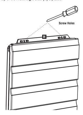
**b** Drill a pilot hole (using 1/8" drill bit) in front lower corner at location indicated by screw target.
